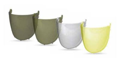
You can choose from two different shade levels 4 and 5 or a bright yellow visor. The brand new toric visors offer excellent optical quality (EN 166 class 1) and enhanced robustness - protection against high-speed particles with HIGH energy guaranteed and against molten metal and hot solids.
