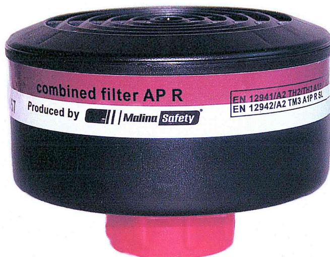
Combined filter flow 105 l/min class TH2/TH3 A1P R SL according to EN 12941/A2 is part of the powered filtering devices CleanAIR Chemical 2F Plus and CleanAIR Chemical 3F incorporating a helmet or a hood and provides protection of respiratory system of user against organic gases and vapours with a boiling point above 65 °C, solid and liquid aerosols, in accordance with the information supplied by the manufacturer.
